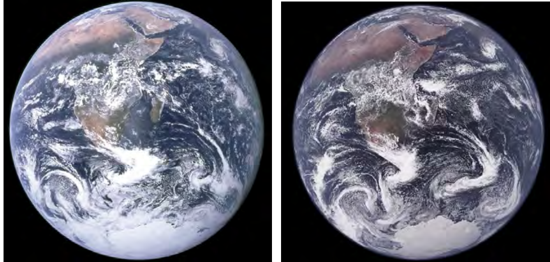
Left: picture from space taken by Apollo 17 astronauts on 7 December 1972. Right: Simulated visible satellite image from a 1.25 km resolution simulation of the ICON model initialized with reanalysis fields on 5 December 1972 by NVIDIA., WMO Bulletin vol 7(29, 2023)
